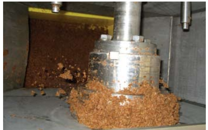
Screw presses use less energy and generate higher total solids than centrifuges.
